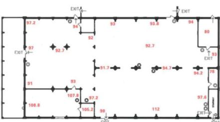
A noise map allows the HCP team to identify noise levels that contribute to a worker's cumulative exposure and indicate where noise reduction efforts are needed.
