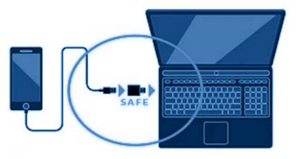
Figure 1. Prevent unwanted data access with a USB data blocker when charging a phone.
